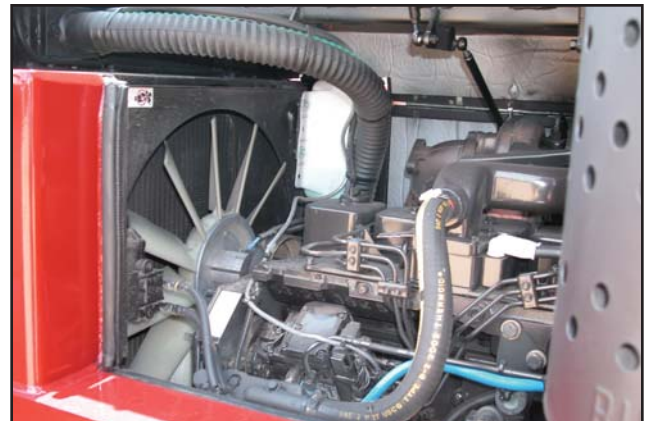
Tier II certified Cummins QSB5.9-30, electronic turbocharged diesel engine
